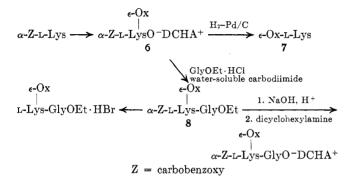
preparation of  $\epsilon$ -Ox peptide derivatives. The diprotected lysine derivatives could be coupled without difficulty and either the carbobenzoxy or ester groups removed in excellent yield in the presence of Ox protection. Cleavage of the protecting groups under the usual conditions afforded L-lysylglycine hydrochloride in excellent yield.
